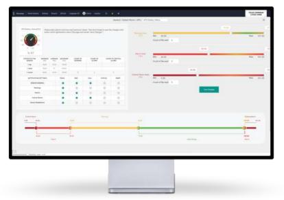
You can receive data from your SNMP/Modbus supported devices through Sensaway Management Software, as well as specify alarm threshold ranges for each parameter separately. You can customize your notifications (mail, SMS, call, syslog, SNMP trap) by creating alarm scenarios according to these alarm thresholds.
